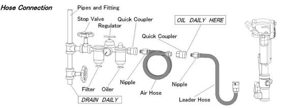
Whether there is any dust, or damage to the air connection portion. Whether the air hose is tight enough.
